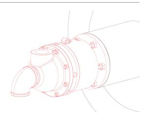
Pay special attention to concentricity. At high speeds the bearing will yield longer, trouble-free service if runout is kept to a minimum.
