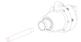
**Important:** Check the pipe is straight and true to prevent excess wear and breakage.
