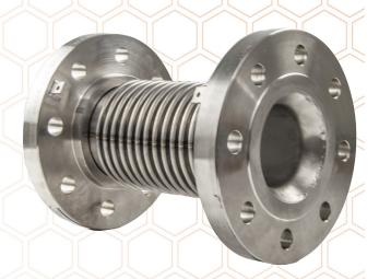
Custom-engineered single- and dual-bellows designs made from 18-8 stainless steel alloy 321 as well as special alloys including Monel, Inconel, and Hastelloy. Options include PTFE-lined, universally-tied, in-line pressure-balanced, externally-pressurized, Gimbal, and hinged, among other configurations. With a wide range of metals, Kadant Unaflex metal bellows expansion joints can be designed to operate up to 300 psi and with temperatures up to 1,500° F in sizes from 2" up to 144".
