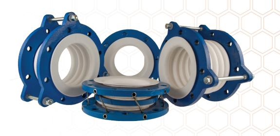
Kadant Unaflex Styles 112A, 113A, and 115A solid-molded PTFE expansion joints are corrosion-resistant and made to withstand the high-pressure and temperature in a compact, space-saving design. Standard sizes from 1" to 12" with two, three, or five convolutions; available in sizes up to 48". Kadant Unaflex PTFE expansion joints can operate with from a full vacuum to 160 PSI depending on the type and number of convolutions.
