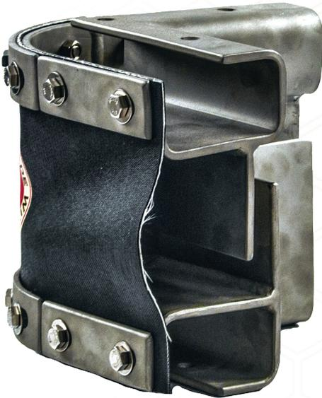
Therma Flex expansion joints are non-metallic flue duct expansion joints or flexible connectors which provide stress relieve for piping and ducting systems by absorbing thermal growth and shock, isolating mechanical vibration, and allowing for misalignments.
