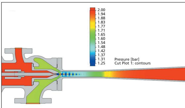
As the motive jet accelerates the suction flow, a low-pressure region is created at the entrance to the mixing chamber. As the flow moves along the mixing chamber, pressure rises. At the diffuser, velocity decreases and pressure rises.
