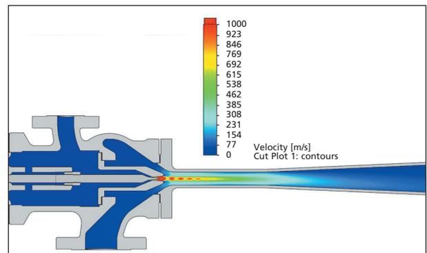
The motive flow is accelerated at the nozzle and a high-velocity jet is created. The jet transfers momentum to the suction flow and accelerates it as the two flows mix.
