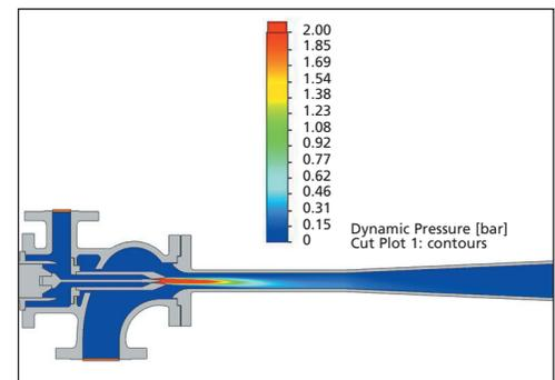
*Velocity head in the mixing chamber with standard geometry.*
