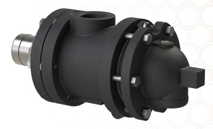
The ELS (Extended Life Series) rotary joint is a self-supported joint that has been specifically designed to solve accelerated wear problems that occur with conventional self-supported rotary joints – particularly those in high vibration applications. The double-guide design provides internal support for the joint and maintains alignment even when the roll or cylinder is not concentric.
