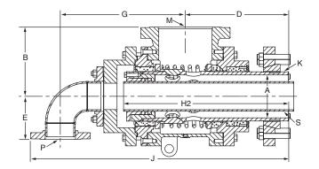
Rotary joint with rotating syphon pipe
