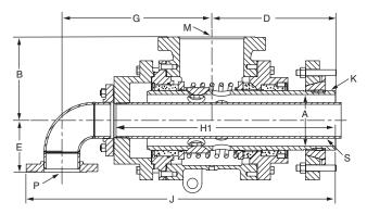
Rotary joint with stationary syphon pipe
