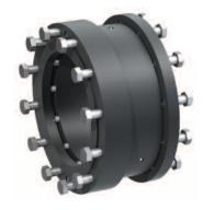
Single-flow passage swivel for door hinge in the municipal waste industry. Features include a recessed and hardened ground shaft and a special bronze bearing for reduced friction.
