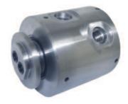
Two-passage, stainless steel rotary union for use on a deionised water application in the semiconductor industry. Designed with a special key-way drive, the rotary union provides a 90 degree swivel movement in 0.3 seconds and cycles every 7 to 30 seconds.
