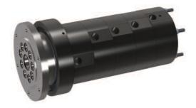
Multi-purpose, ten-passage, flange mounted rotary union for the tire industry. Features include a recessed and hardened ground shaft, through-bore to accommodate an additional rotary union, and deep groove radial contact bearings.
