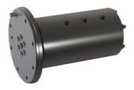
Multi-purpose, seven-passage, flange mounted rotary union for the tire industry. Features include a recessed and hardened ground shaft, through-bore to accommodate an additional rotary union, and deep groove radial contact bearings.
