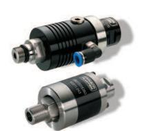
The  $G^{TM}$  high precision rotary unions are generally applied to spindles on CNC machines, gun drilling, milling, and other machinery. These rotary unions are designed for speeds up to 50,000 RPM and pressures up to 250 bar (3,600 psi) in sizes ranging from m10 ( $\frac{1}{4}$ ") to m16 ( $\frac{5}{8}$ ").
