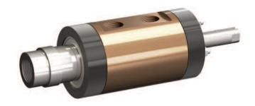
Multi-purpose, two-passage, thread mounted rotary union used for mixing glass in liquid fusion. Features include a recessed and hardened ground shaft and deep groove radial contact bearings.
