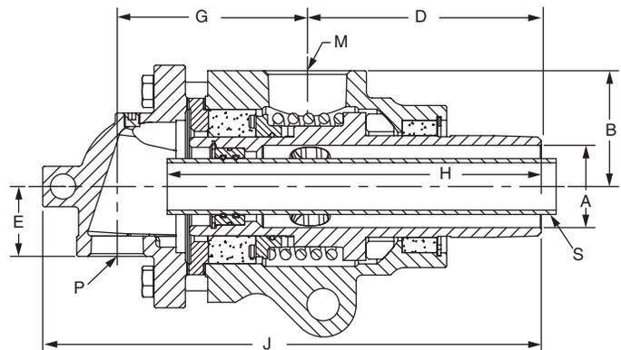
4" SNX Rotary Joint Shown with Packing Seal Option.
