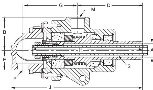
3" SNXA Rotary Joint Shown with O-ring Seal Option.
