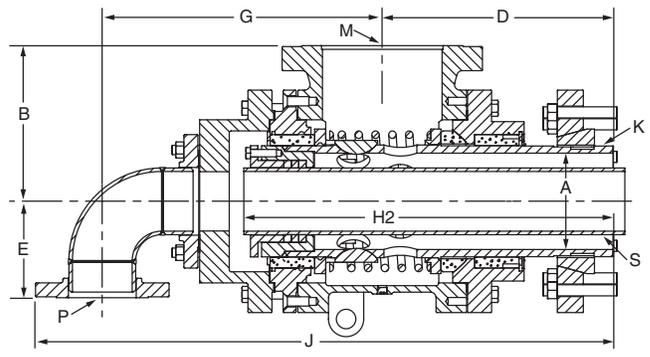
Rotary joint with rotating syphon pipe
